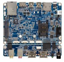
Powered by WM8950 Cortex A9 Single-Core 800MHz processor
