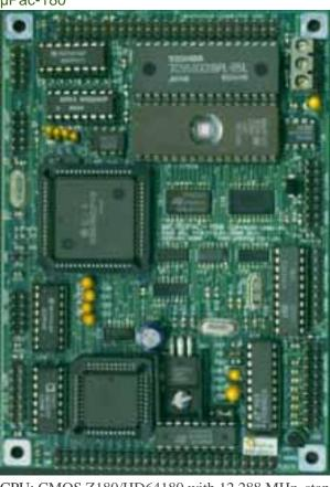
CPU: CMOS Z180/HD64180 with 12.288 MHz. standard crystal speed.
