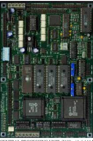
CENTRAL PROCESSING UNIT: Z180 with 6.144 MHz clock speed.
