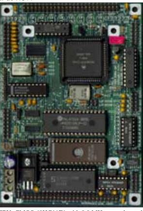
CPU: CMOS 68HC11F1 with 8.0 MHz crystal speed
