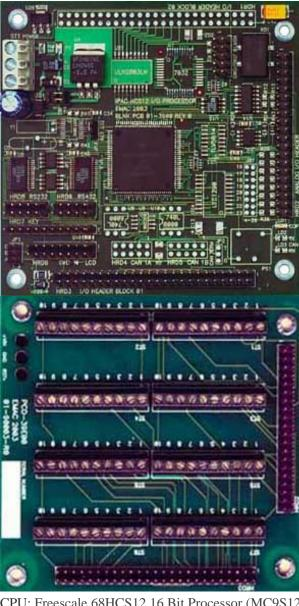
CPU: Freescale 68HCS12 16 Bit Processor (MC9S12DG256BCPV) running with a CPU clock speed of about 50 MHz with BDM debugger capability.
