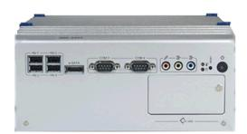
Intel® Atom<sup>TM</sup> D510/D525 dual core up to 1.8 GHz fanless embedded IPC
