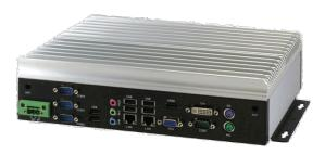
Intel® 32/45nm Core™ i7/i5/i3 rPGA988 CPUs With Graphic& Memory Controller
