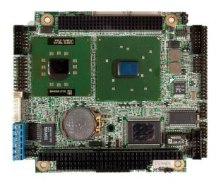
Intel Ultra Low Voltage Embedded Celeron M or Pentium M Processor
