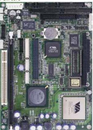
Embedded low power VIA 400 MHz to 1 GHz processor
