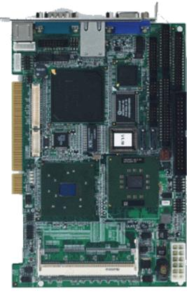
Embedded Fanless Intel Celeron M 600 MHz Processor
