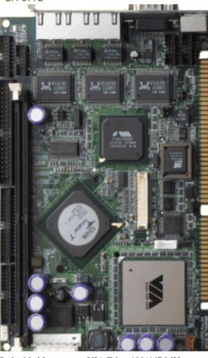
Embedded low power VIA Eden 400/667 MHz
