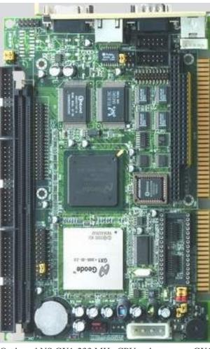
On-board NS GX1-233 MHz CPU or low power GX1-300
