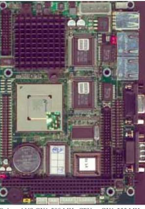
Onboard NS GX1-300 MHz CPU or GX1-233 MHz CPU
