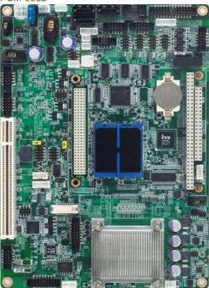
Embedded Intel® Atom Fanless N450 or D510 (Dual Core) Processor
