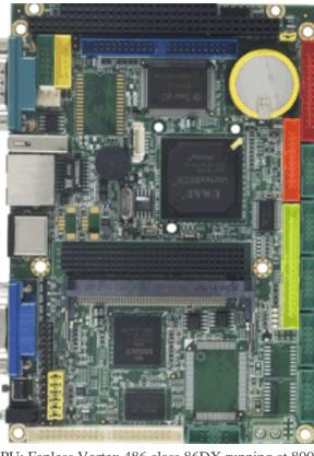
CPU: Fanless Vortex 486 class 86DX running at 800MHz
