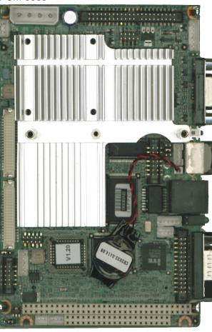
Embedded Onboard Intel® Fanless Celeron® M Processor
