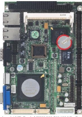
Onboard AMD Geode LX800/900 500/600 Mhz Processor
