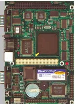
Compact size (145 mm x 102 mm). Fits in the space of a 3<sup>1</sup>/<sub>2</sub>" HDD
