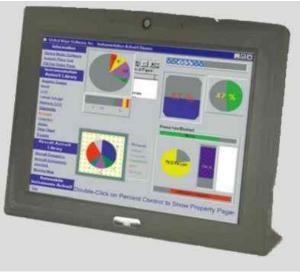
8" LED backlight LCD panel with resistive touch screen
