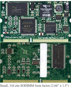
Blackfin hybrid RISC/DSP high performance core running at up 600 MHz
