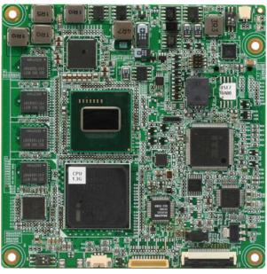
Onboard Intel Atom E680 Processor
